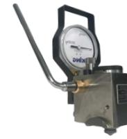
**STANDARD TEST HEAD** - Loads of 3000 kgf, 1500 kgf Provides reliable and accurate results.
