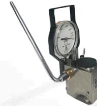
**LOW PRESSURE TEST HEAD** - Lower pressure test for softer metals loads of 62.5 kgf, 125 kgf, 250 kgf, 500 kgf, 750 kgf or 1000 kgf.
